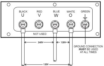
Figure 29. Output Terminal Lugs 1Ø-240/120V Connections
